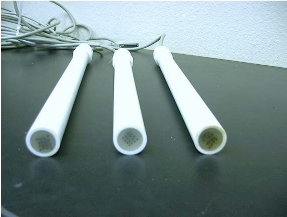
Figure 2. Typical 16-electrode MAS probes used in the experiment
