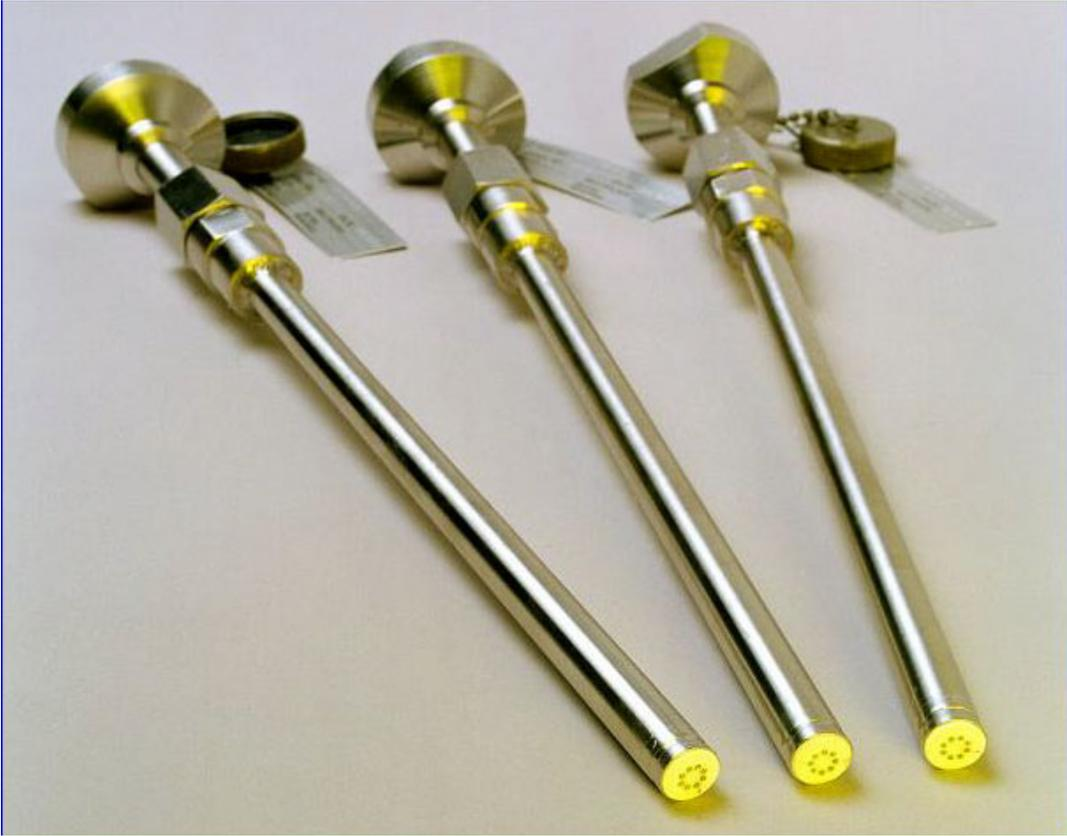
FIGURE 1. Coupled multi-electrode array sensor (MAS) probes for application in a pressurized process stream at elevated temperatures
